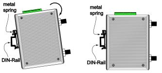
To remove the AWK-3121 from the DIN-Rail, simply reverse Steps 1 and 2.
