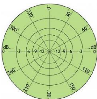
TYPICAL RADIATION PATTERN (H-PLANE)
