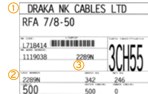
Drum label shows 1 cable type 2 length 3 gross weight 4 batch number
